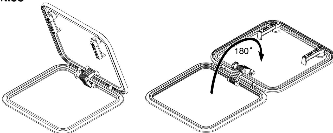
The hatch can be opened to a maximum 180 degree angle. Please ensure there is sufficient room when fully opening the hatch to 180 degrees.
